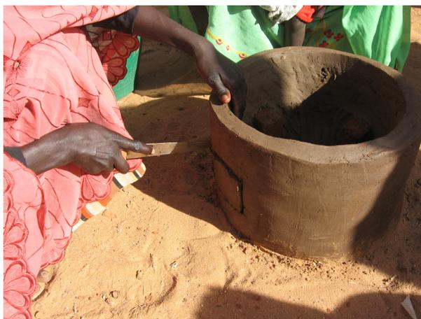
Figure 3: Cutting the hole for fuel access. This needs to be large enough for wood and ventilation. Photo: Practical Action, Sudan.
